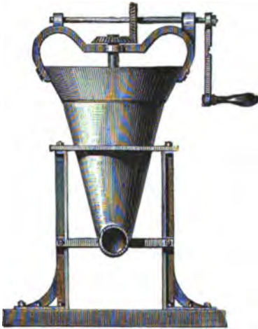
Fig. 396.—Gysser's machine for pressing peat.
